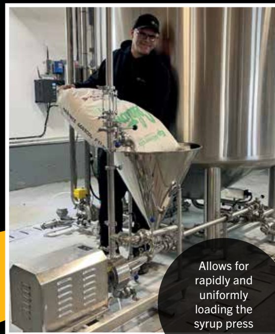
Dynamic Mixer YRL 1-100 with 5.5 HP motor 668429
